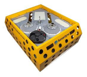
Origin<sup>®</sup> Seabed Lander is a dedicated solution that can integrate everything you need to support your Origin 600 Acoustic Doppler Current Profiler (ADCP) operations. It simplifies deployments by integrating Origin 600, Origin E-Mux, Origin PowerPlus, and up to four thirdparty sensors into one compact payload. Two acoustic releases are integrated as standard for dual redundancy.
