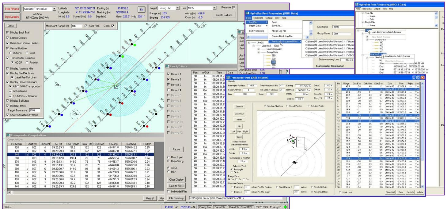
**HydroPos version 3 is a software programme that works with Sonardyne’s Ultra Short Baseline (USBL) Mini-Ranger 2 (HF) and Ranger 2 (MF) systems as well as the Transition Zone Transceiver (TZZ – MF & HF). It enables multiple transponder locations to be tracked automatically selecting the transponders to be interrogated as the vessel sails along the deployed seismic receiver cables or nodes.**
