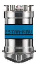
Lodestar-Nav 200 provides all-in-one navigation for subsea vehicles and survey operations by combining solid state Attitude Heading Reference System (AHRS), a Syrinx Doppler Velocity Log (DVL) and a high accuracy pressure sensor in a single housing. The Lodestar-Nav is upgradable to SPRINT-Nav Acoustically Aided Inertial Navigation System [AAINS].
