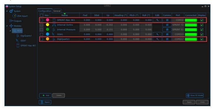
The desired depth sensor should be selected for use in the appropriate solution in the Navigation Solutions configuration window:
