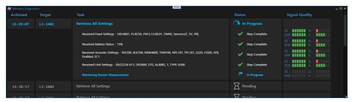
If an acoustic telemetry task fails, the user can choose to skip, retry, or cancel the task.
