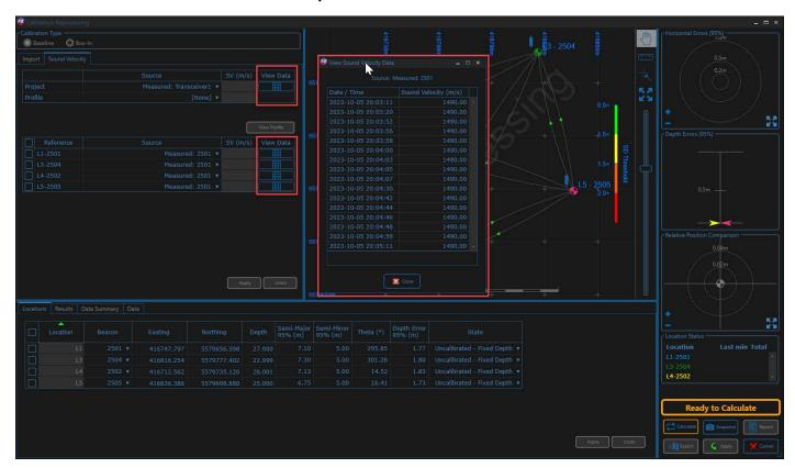
35045 Provide Ability to Select a Different Sound Velocity Source Configuration per Calibration Dataset
