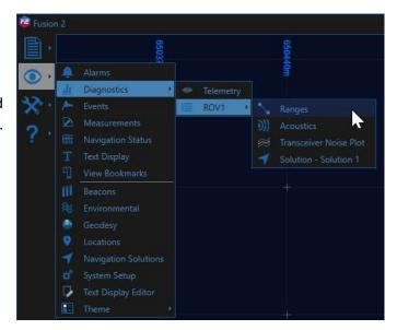
The tool displays information about each acoustic range which is expected to be received by the transceiver on the selected vehicle, and their use in the selected positioning solution. The solution for which information is displayed can be changed using the drop-down menu at the top of the tool window.
