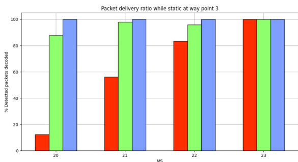
Fig. 3 - Packet delivery rates for 24kHz static signals in Plymouth Sound (red trace RC, green trace AR, blue trace 6-channel AR, BT16,32,64,128 left to right) [3]
