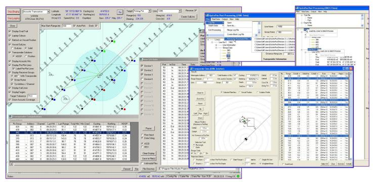
HydroPos Version 3 is a software programme that works with Sonardyne's Ultra Short Baseline (USBL) Mini-Ranger 2 (HF) and Ranger 2 (MF) systems as well as the Transition Zone Transceiver (TZT – MF & HF). It enables multiple transponder locations to be tracked automatically selecting the transponders to be interrogated as the vessel sails along the deployed seismic receiver cables or nodes.
