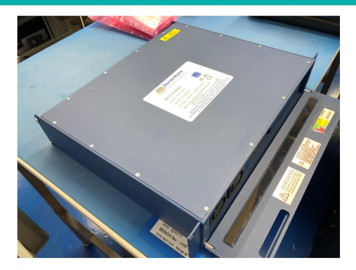
3. Remove the lid and remove the dongle.
