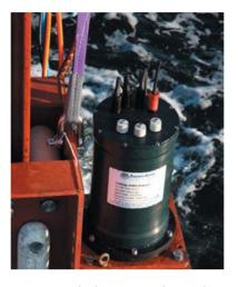
As a stand alone unit, the Lodestar AHRS provides precise readings for vessel heave, heading, roll and pitch with negligible latency. Due to the high quality accelerometers and gyroscope elements in Lodestar, the unit is capable of significantly outperforming traditional survey grade sensors.
