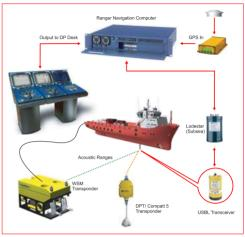
A high speed Ethernet link between the Lodestar AHRS and Ranger USBL computer ensures fast data transfer and zero latency, resulting in a further improved USBL position solution output to the survey team and/or DP desk.
