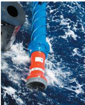
GyroUSBL was deployed on an Over-The-Side deployment pole fitted to the vessel HOS Sweetwater .
