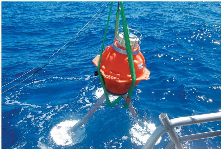
PIES can be free fall deployed to the seabed where it will land in an upright position.
