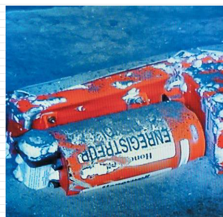
One of the flight data recorders recovered from the seabed, it was located by a Remora 6000 ROV tracked using a Ranger 2 USBL. (Photo: BEA).
