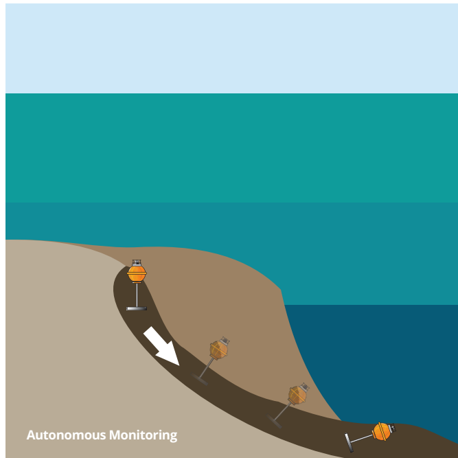
Above, left: Instruments used to measure underwater avalanches have to be able to live through major displacements. Above right: Plate tectonic measurement has been boosted by GPS-A techniques.
