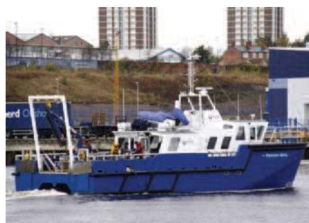
(Clockwise) Sea acceptance trials were conducted off the coastal town of Bridlington, Yorkshire. Figure 1 Solstice sonar image of a leak target with a flow rate of 15 litres per minute. The SAT was led by Fugro from the RV Princess Royal, a 19 metre catamaran specifically designed for marine environmental surveys.
