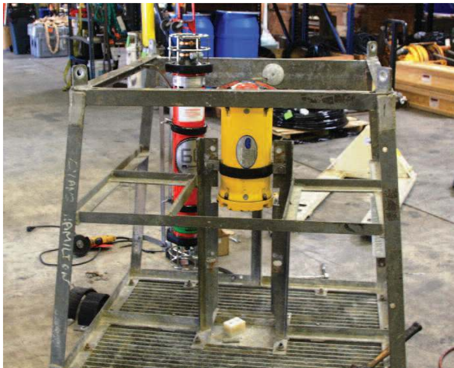
(Opposite page) A Sonardyne HPT Modem configured for cable deployment from over the side of the rig. A cage provides protection from potential damage whilst weight behind it minimises drifting in surface currents. (Left)
