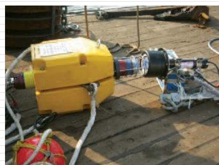
(Clockwise) Looking back to 2007 with NIOT's deployment crew and one of the first surface buoys ready to be installed. Cleaning marine growth from surface transceivers is undertaken during regular service visiting to each station. In air acoustic deck testing of a BPR is carried prior to deployment.
