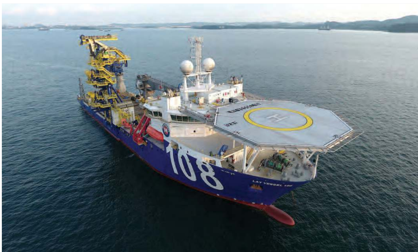
McDermott's LV 108 entered service in 2015 and is currently on contract in the Ichthys field, Western Australia. Designed as a fast-transit, dynamically positioned (DP 2) vessel for subsea construction support across a wide variety of water depths, the LV 108 can accommodate a crew of 129.
