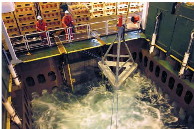
(Left to right) AMTs in frames deployed easily and quickly from a vessel's moon pool; Section of transponder locations including lines of sight between each unit; Spiked AMT frame allows transponders to be deployed on small ridges without fear of movement whilst collecting data; Transceiver deployed on an over the side deployment pole from a vessel of opportunity to collect data.
