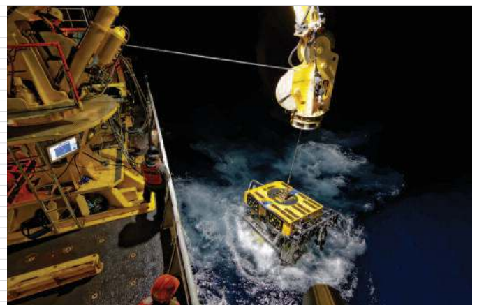
Deploying ROPOS, a free-flying 4,000 metre ROV. Image: © Ed McNichol
