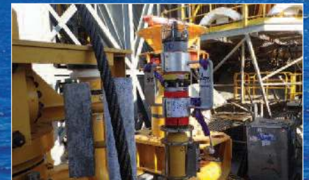
Real-time positioning and heading information was gathered by a GyroCompatt and streamed to SensorView on the surface.
