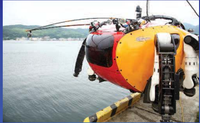
(Above) Crabster is an autonomous walking and flying crab-like robot being developed by KRISO's ocean systems engineering department. (Below) BlueComm data rate and range performance comparison.
