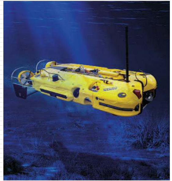
Saab Seaeeye's Double Eagle SAROV, fitted with Solstice high resolution imaging sonar, being deployed on mission. (Below) Solstice is a low-power, compact side-scan sonar that uses full dynamic focus and multi-ping techniques to gather high fidelity imagery fully corrected for vehicle motion.
