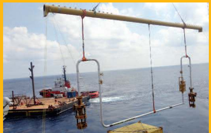
(Top) Sonardyne 6G LBL based acoustic metrology provides the best level of accuracy and QC and is the reference against which all other methods are compared.
