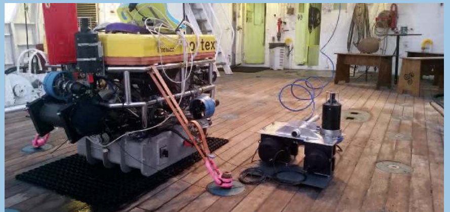
Vortex is Ifremer's demonstration and test bed Hybrid ROV which BlueComm was fitted to for the trial. Equipped with a 3800 Wh battery Vortex could operate remotely via a WiFi link for over 4 hours. The WiFi link is provided by a tethered buoy which floats on the surface as Vortex dives to depth. A configurable on board camera provides high bandwidth data to test the BlueComm link.
