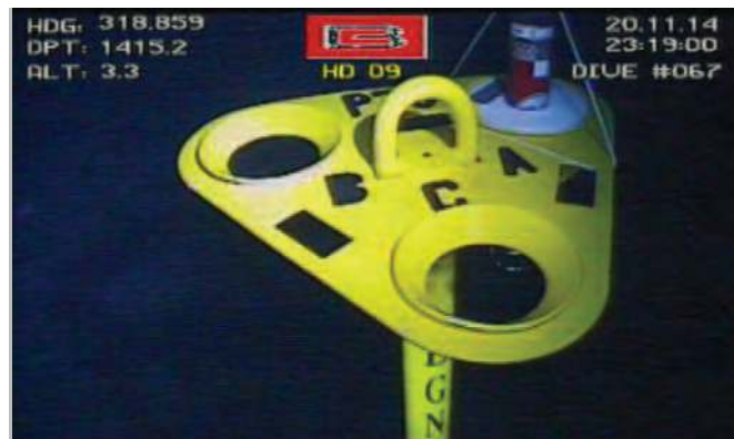
(Above and left) A Sonardyne Compatt 6 transponder that forms part of the field-wide acoustic positioning network at the Egina oil field, is lowered to the seabed. Compatt 6 is the industry standard LBL transponder used for high precision subsea survey and construction operations in all water depths.
