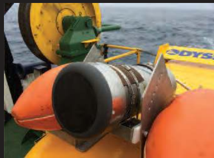
Odyssey's new deep tow platform, equipped with an upward looking GyroiUSBL, was tracked to beyond 7,500 metres during trials in the Bay of Biscay.
