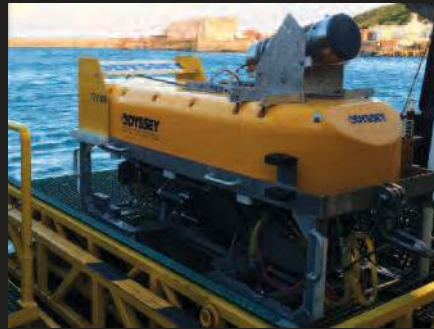
Odyssey's new deep tow platform, equipped with an upward looking GyroiUSBL, was tracked to beyond 7,500 metres during trials in the Bay of Biscay.
