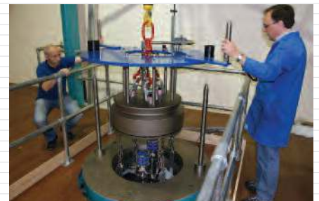
(Above) Commissioning of a new deep rated pressure chamber and 3-axis motion simulator (below).
