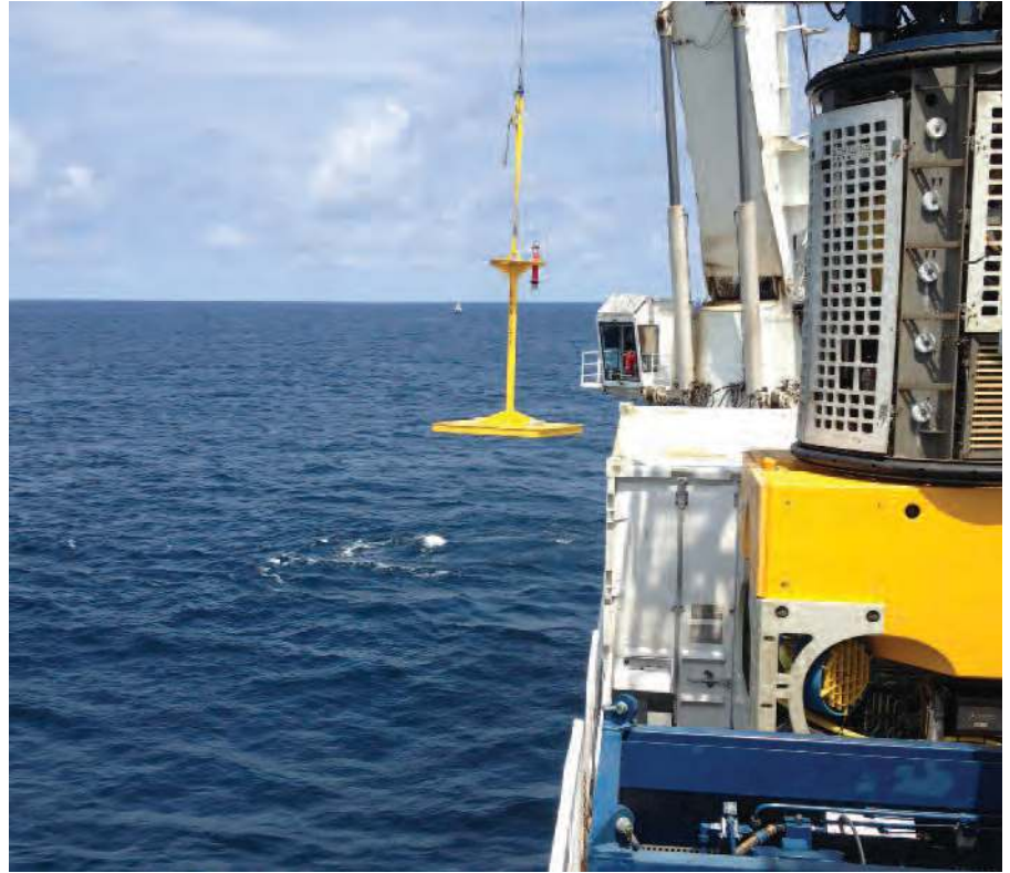
(Above and left) A Sonardyne Compatt 6 transponder that forms part of the field-wide acoustic positioning network at the Egina oil field, is lowered to the seabed. Compatt 6 is the industry standard LBL transponder used for high precision subsea survey and construction operations in all water depths.
