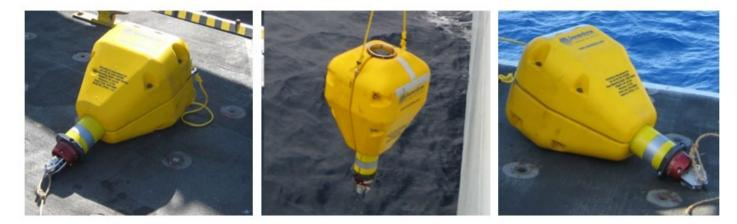
Subsurface floatation collars enable acoustic navigation and positioning transponders to be deployed, moored on the seabed and then recovered to the surface.
