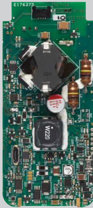
Transducer and PCB shown actual size (56 millimetres x 88 millimetres)
