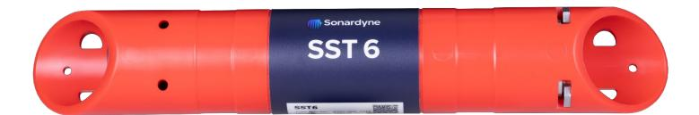
The Type 8325 Small Seismic Transponder 6 (SST 6) is a small rugged transponder designed for acoustic positioning of ocean bottom seismic cables and nodes, where high-performance, small-size, low-cost and ease of programming are all important operational factors.
