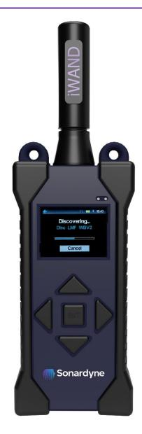
The iWand is a handheld acoustic transponder test and configuration device developed for use with Sonardyne's 6G® product range.
