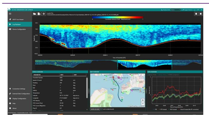
Echo Observer for Syrinx (EOS) is a software application for Syrinx and SPRINT-Nav systems allowing Acoustic Doppler Current Profiling (ADCP) data to be viewed, quality controlled, logged, and then exported.
