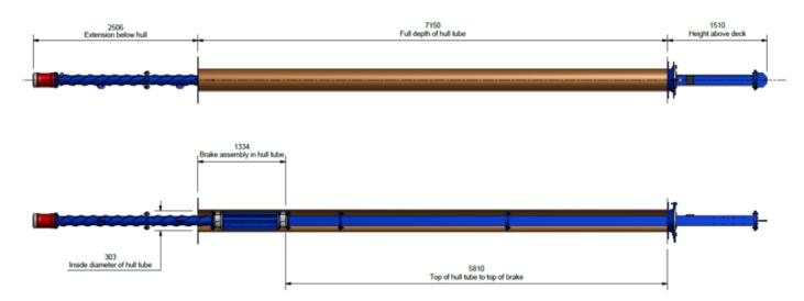
Dimensions will vary depending on vessel. The above is suitable for a vessel with a 7.5 metre tube.
