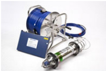
Cable drum, SIU and Dunker
